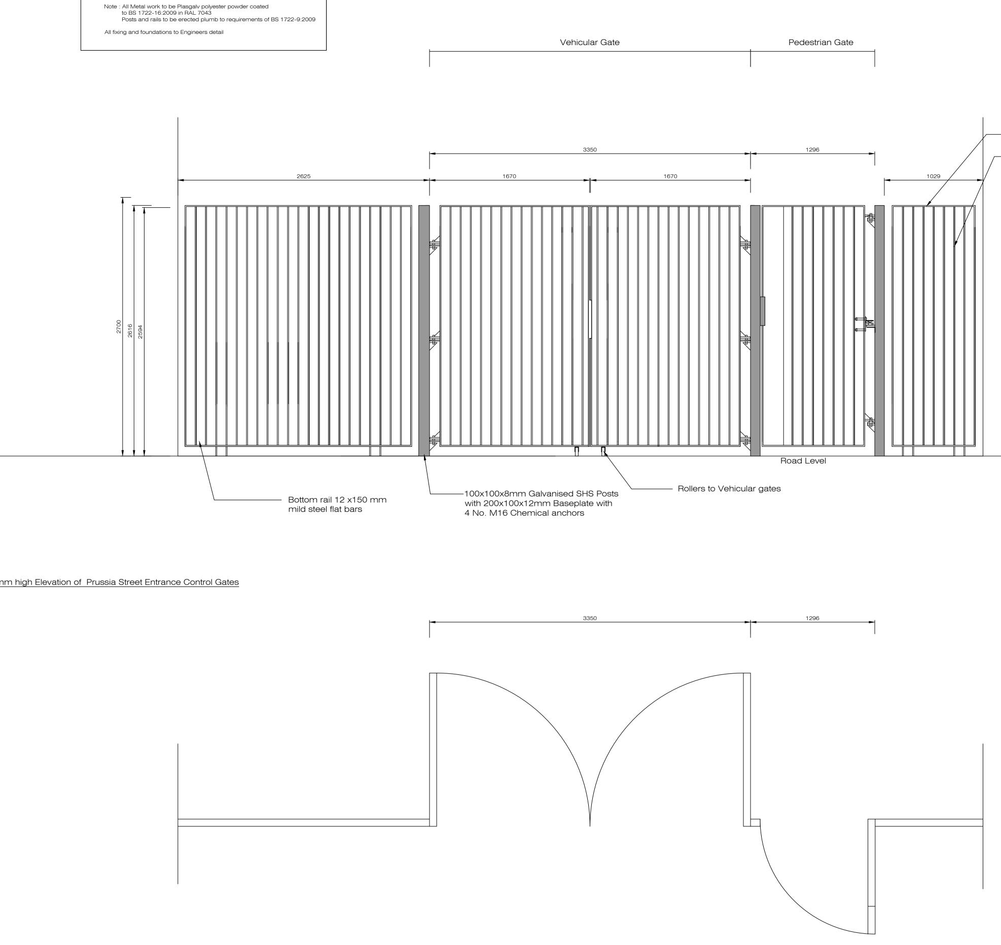
Detail 01 LD-03-PP 2500mm high Elevation of Prussia Street Entrance Control Gates Elevation Scale @ 1:20
